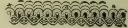
Section of Brussels Carpet. Loops woven over wires A; B, wires removed.
